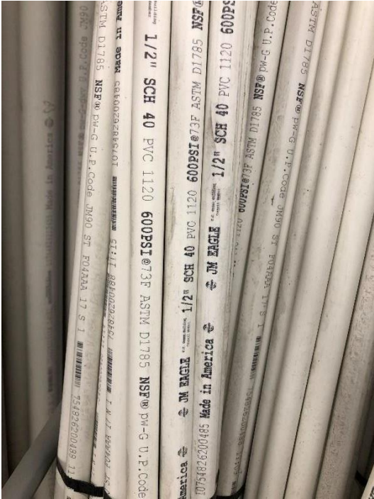
Potable white PVC line with NSF label
