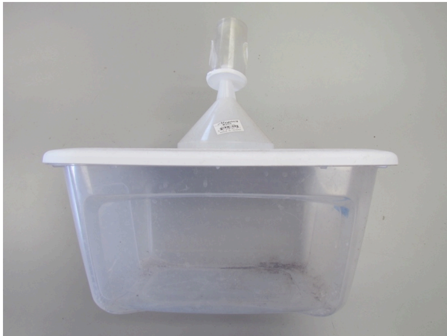
Figure 6. Fourteen-quart clear plastic tub used for monitoring emergence of eye gnats from soil samples. A hole was cut on the lid with an inverted funnel glued to the top. A 40-dram vial is attached to the spout of the funnel to collect emerged adult gnats.
