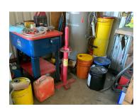
Inspector note: <10 gallons of flammable combustible liquids found in the hangar at time of inspection. Storage amount poses imminent hazard to the building. Immediately dispose excess amount or store in flammable cabinet(s).
