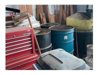
Inspector note: Store excess of 10 gallons of flammable/combustible liquids inside flammable cabinet(s) or remove from hangar. Violation is due to be rechecked on 06/01/2021
