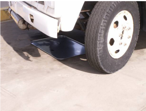
A temporary drip pan is placed under a vehicle.
