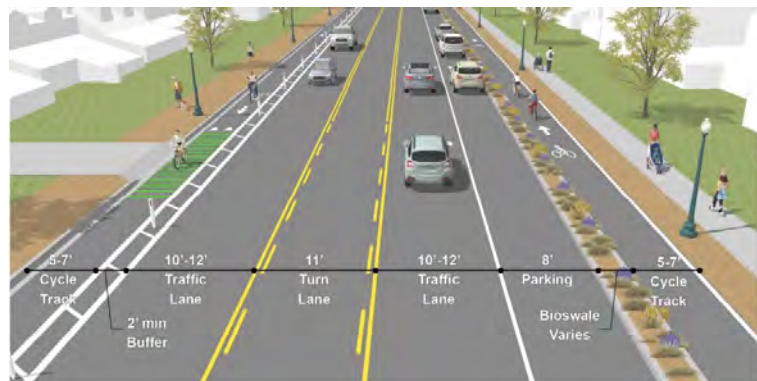
Figure 11: Class IV Separated Bikeway (Source: County of San Diego Active Transportation Plan , 2018. Appendix B Toolbox)
