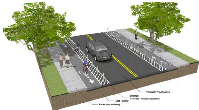
Figure 4: Illustration from County of San Diego ATP, Class IV Bikeway with Bollards Concept (referred to as flexible delineator posts in the concept development)
