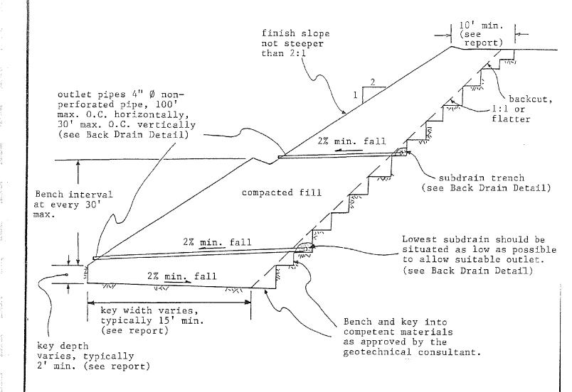
Notes: For buttress dimensions, see geotechnical report/plans. Actual dimensions may be changed by the geotechnical consultant based on field conditions.
