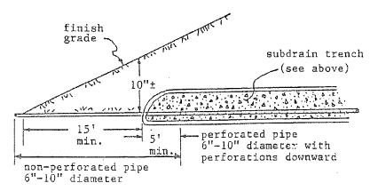
NOTE: Subdrain to be installed in competent material as evaluated by the field representative. Non-perforated pipe to be installed in regions recommended by the field representative.
