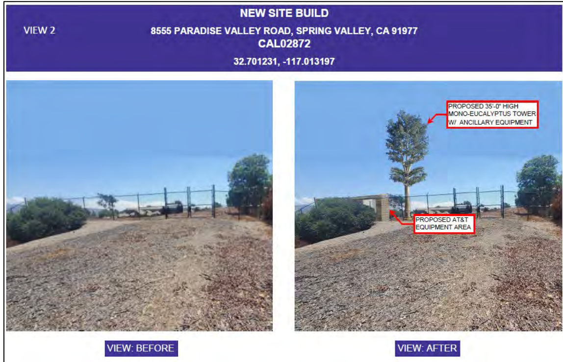
Figure 2: Photosim of proposed mono-eucalyptus tower and proposed AT&T equipment enclosure (north of project site)
