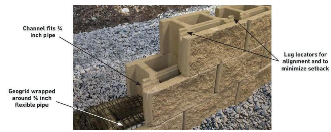
6 RETAINING WALL - IMAGE FOR REFERENCE ONLY SCALE: 3/8" = 1'-0"
