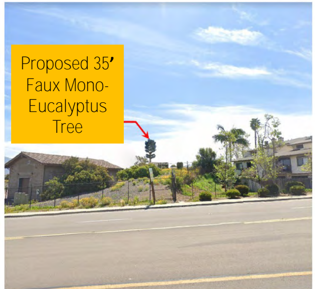
Figure 2: Photosim of proposed mono-eucalyptus tower and proposed AT&T equipment enclosure (north of project site)
