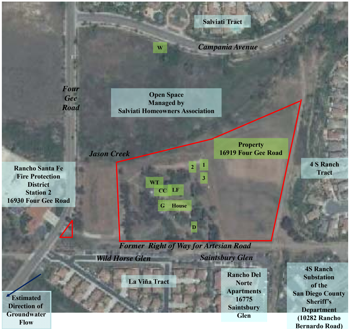
FIGURE 2 - PROPERTY PLAN Base aerial photograph dated June 4, 2016. Approximate Scale: 1" = 250' North Legend: CC = Caretaker's Cottage D = Dumpster G = Garage LF = Leach field W = Water well WT = Water tank 1 = Remnants of barn pad 2 = Location of former Be Wiser Ranch ASTs 3 = Remnants of Be Wise Ranch cold storage pad
