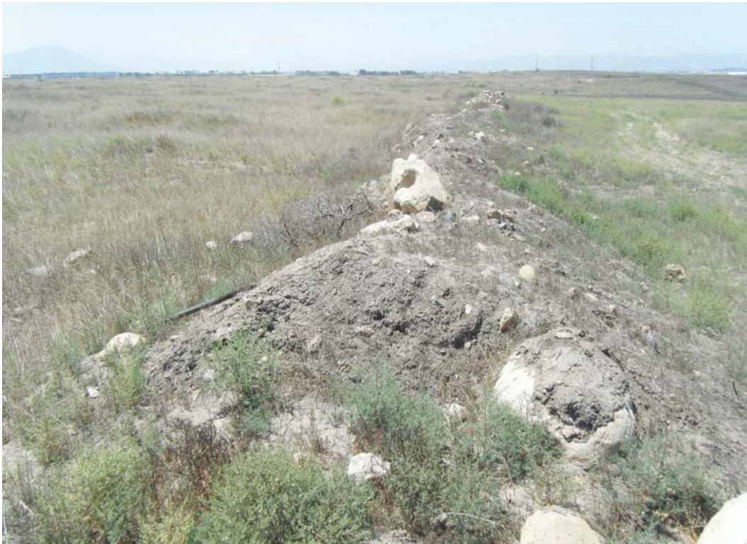
2) View of re-worked native soil from road grading at the northern portion of the Site.
