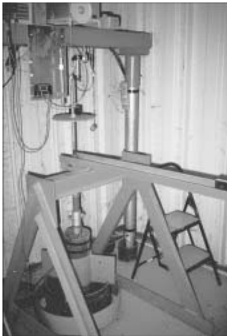
Figure 19 Photograph of extensometer
