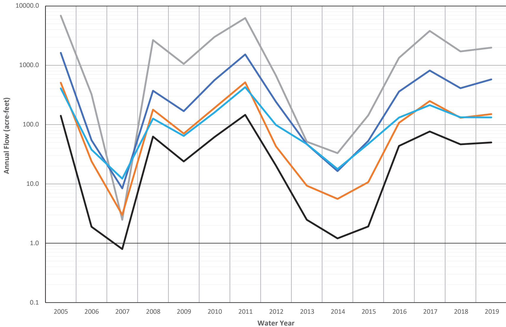
FIGURE 3-25 Groundwater Recharge in Contributing Catchments Computed with the BCM Numerical Flow Model Documentation San Pasqual Valley Groundwater Basin Groundwater Sustainability Plan San Pasqual Valley, California
