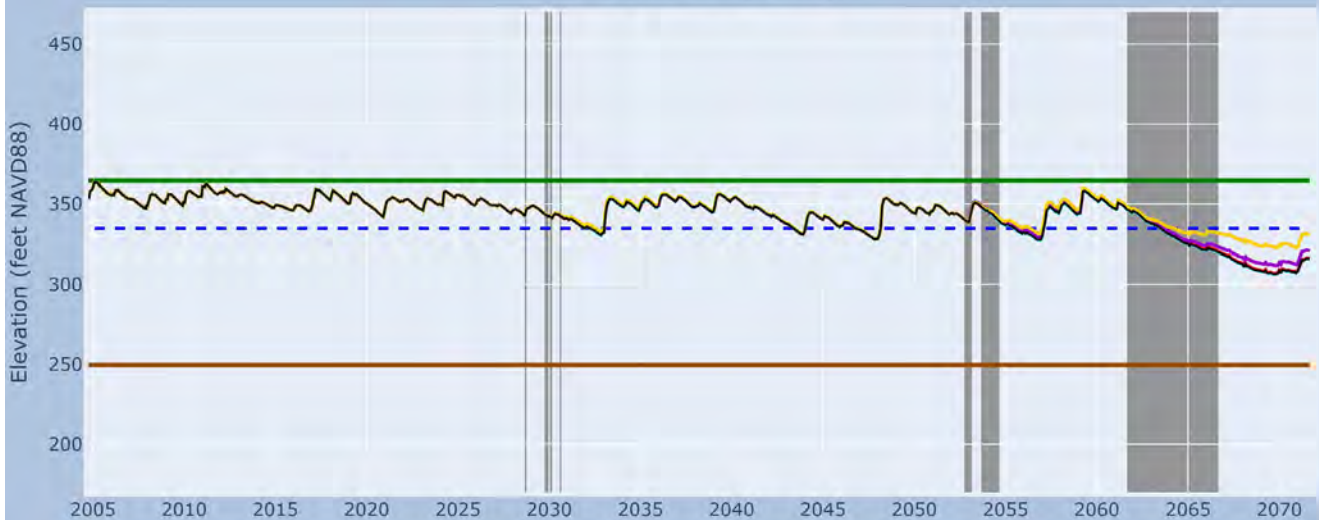
Figure E-7 Recharge Strategy Groundwater Level Hydrographs PMA7: Initial Surface Water Recharge Evaluation Task 5 Groundwater & Surface Water Simulations San Pasqual Valley, California
