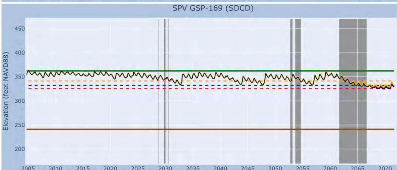
Figure E-4 Recharge Strategy Groundwater Level Hydrographs PMA7: Initial Surface Water Recharge Evaluation Task 5 Groundwater & Surface Water Simulations San Pasqual Valley, California
