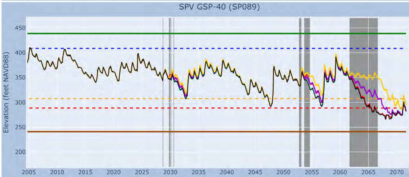
Figure E-1 Recharge Strategy Groundwater Level Hydrographs PMA7: Initial Surface Water Recharge Evaluation Task 5 Groundwater & Surface Water Simulations San Pasqual Valley, California
