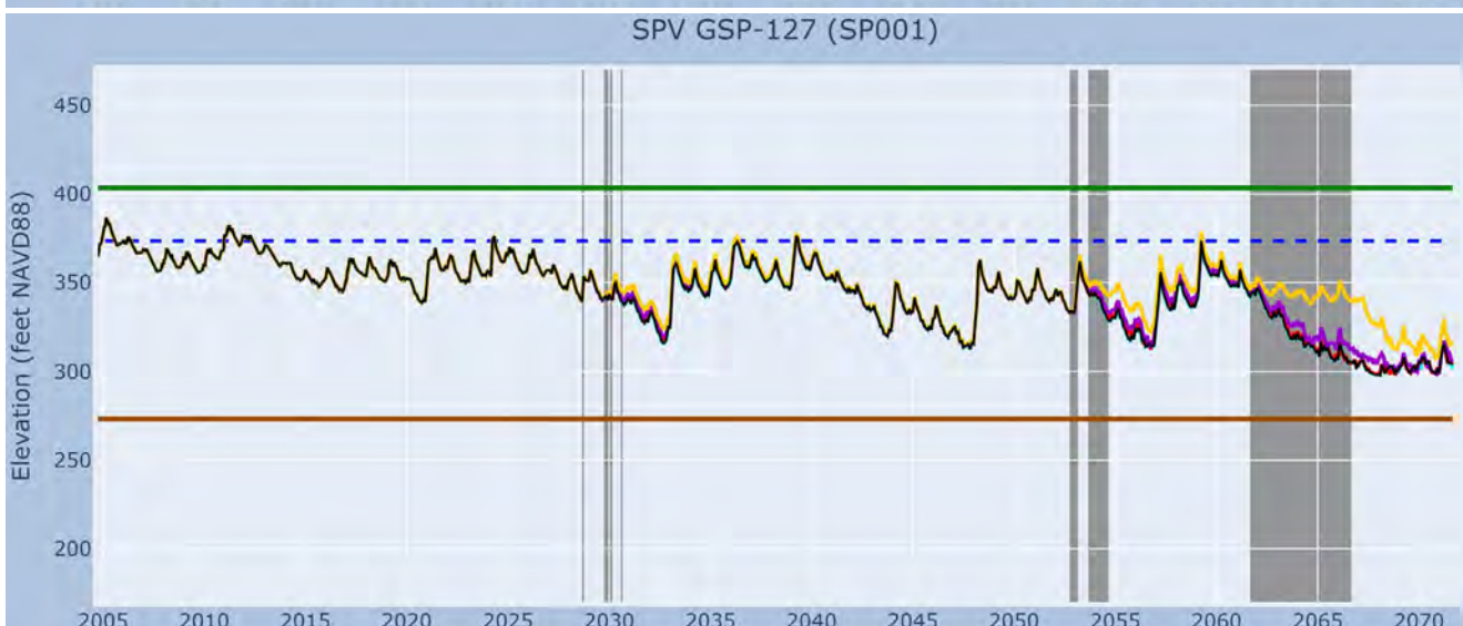
Figure E-6 Recharge Strategy Groundwater Level Hydrographs PMA7: Initial Surface Water Recharge Evaluation Task 5 Groundwater & Surface Water Simulations San Pasqual Valley, California
