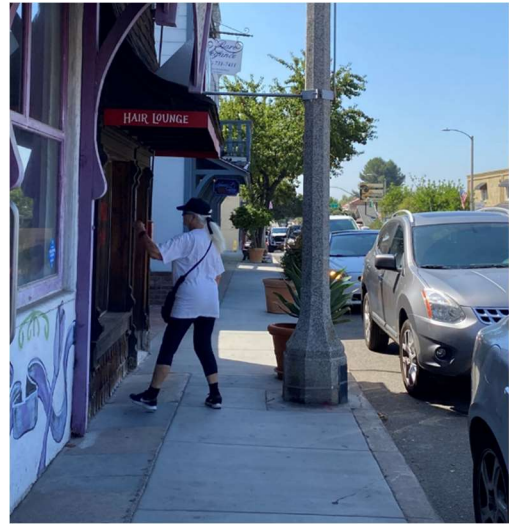
Figure 1: Existing sidewalk on Main Avenue show deficient widths between building and streetlight. (<4 feet)
