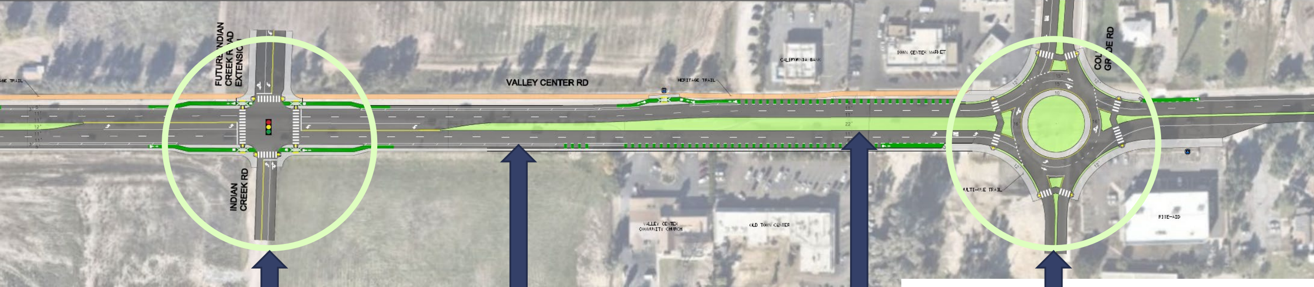
SIGNALIZED INTERSECTION WITH CURB EXTENSIONS
