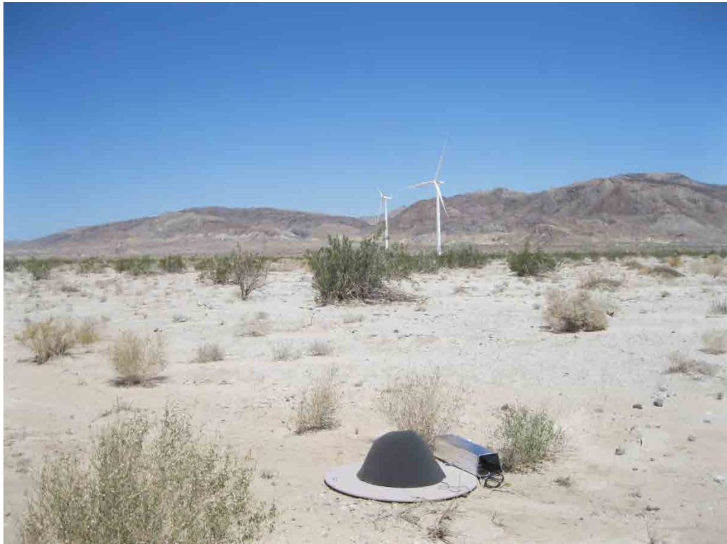
Figure 5 Reference Location O-R2 with Microphone, Ground Board and Windscreen
