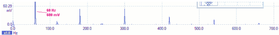
And its corresponding spectrum. Note the relatively few power frequency harmonics.
