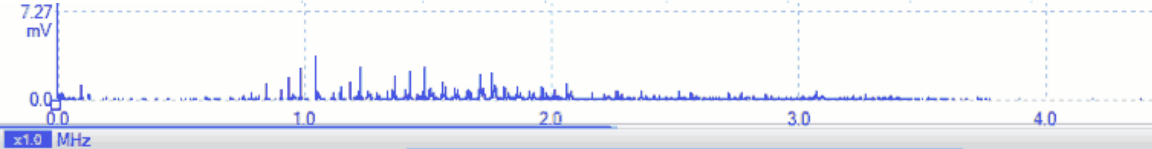
Neutral to Earth voltage with power off – wide-band EMI
