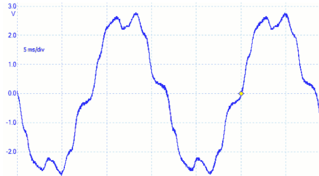
Neutral to Earth Voltage with power off – wide-band EMI
