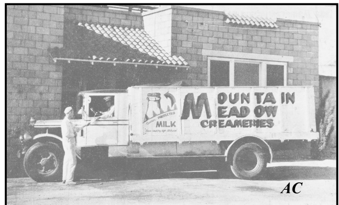
Mountain Meadow creamery has added this General Motors truck equipped with an 1100-gallon stainless steel lined, cork insulated thermos tank to its fleet, for carrying milk from its Jacumba ranch to San Diego in three hours. Milk is maintained at even temperature and is unloaded by forced air pressure. The firm also has added Diveco enclosed type milk delivery trucks.
