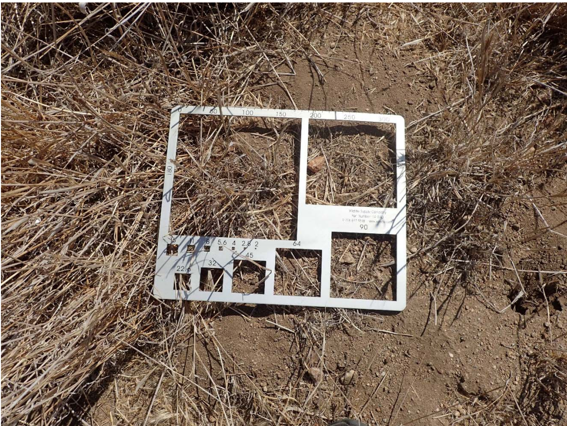
Figure 6. Gravelometer along Reach 2A
