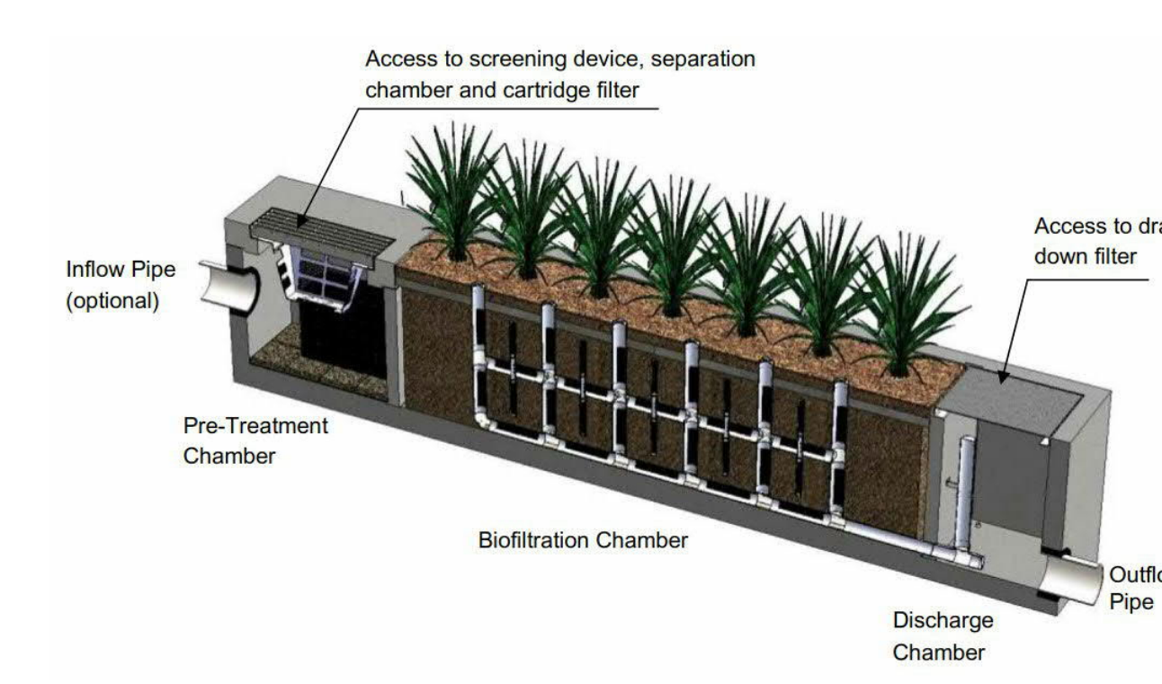
TYPICAL BIFILTRATION UNIT BIO-FILTRATION UNIT AS REFERRED TO IN SWAMP DATED AUGUST 2018 MANUFACTURER, MODEL NUMBER, AND SIZING TO BE DETERMINED IN FINAL ENGINEERING
