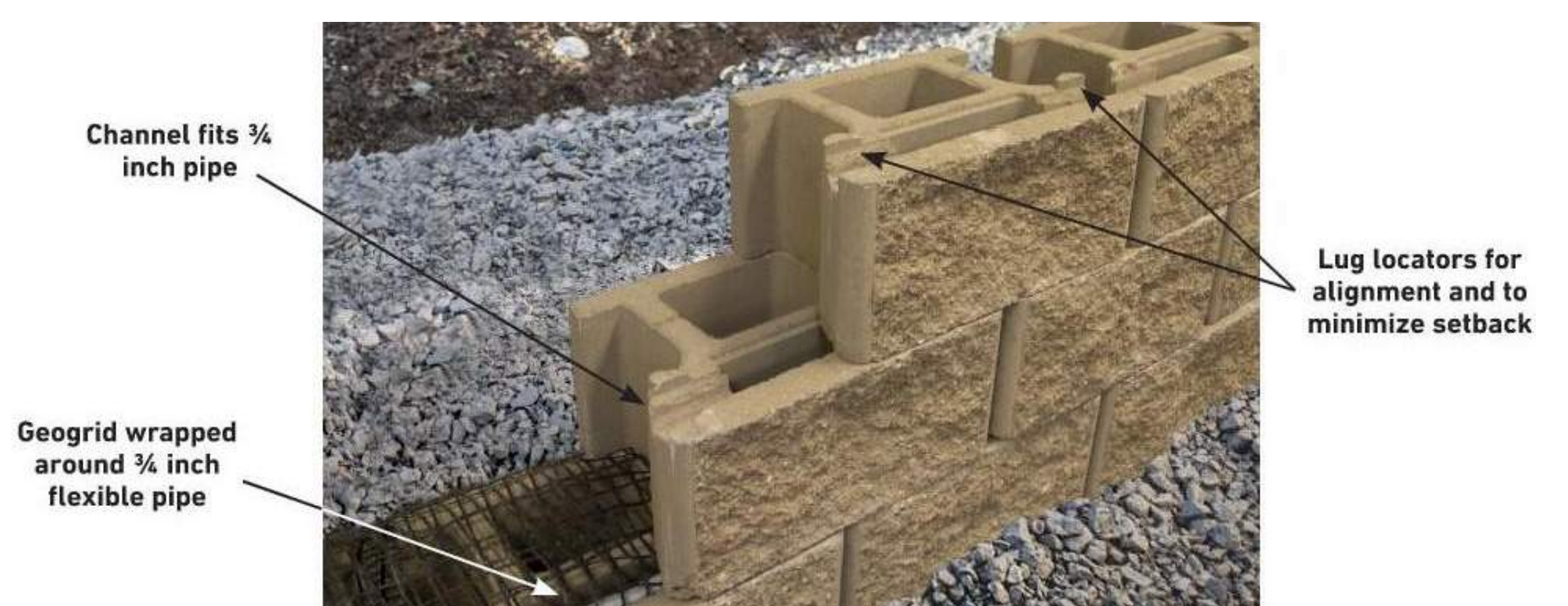
6 RETAINING WALL - IMAGE FOR REFERENCE ONLY SCALE: 3/8" = 1'-0"
