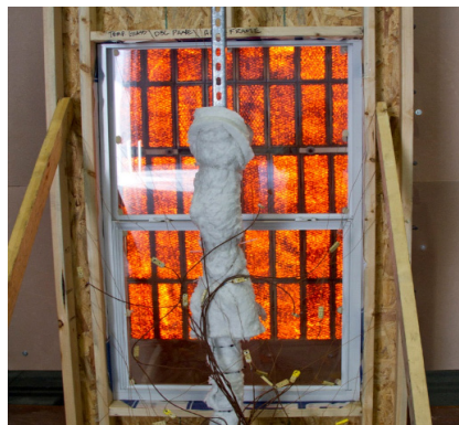
Radiant heat. Here an infrared burner is used to simulate the radiant heat from flame.
