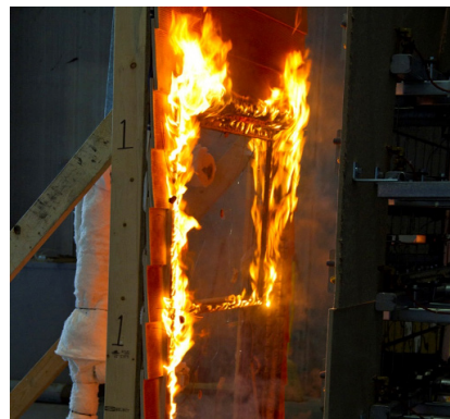
Radiant heat. The radiant heat caused the glass to break and the window frame to ignite.
