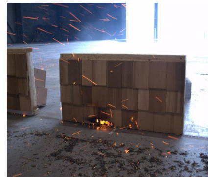
Direct ignition. Embers have accumulated and ignited combustible wood shake siding.
